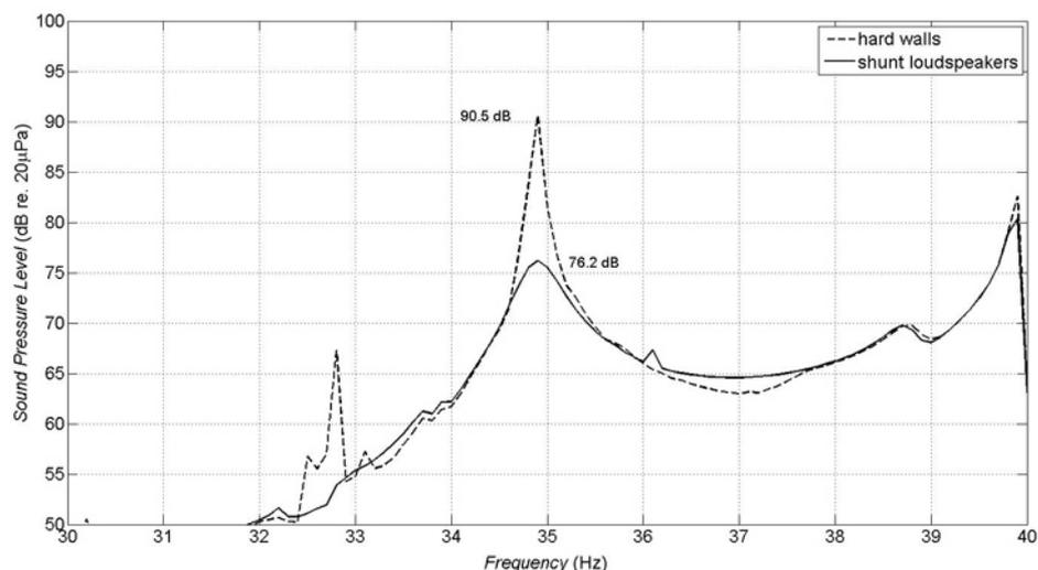
**Figure 6: Stationary sound pressure levels measured in the LEMA reverberant chamber, between 30 Hz and 40 Hz, at corner #4, for 2 different treatments (hard walls and shunt loudspeakers)**
