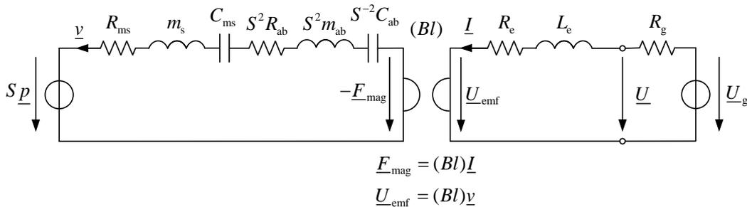
**Figure 2: Circuit representation of generalized closed-box loudspeaker system**
