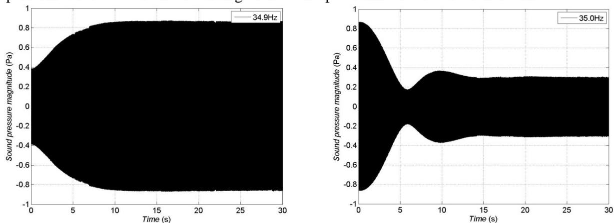
**Figure 7: temporal behaviour of the acoustic pressure in the vicinity of the mode, with hard walls (left: 34.9 Hz; right: 35.0 Hz)**
