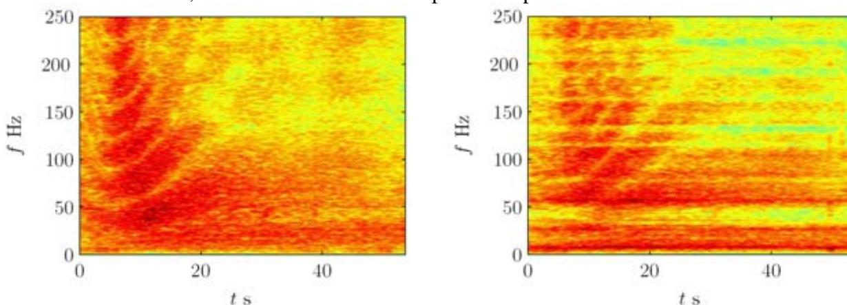
**Figure 1: spectrograph measured during aircraft flyover outside a room (left chart) and inside (right chart).**
