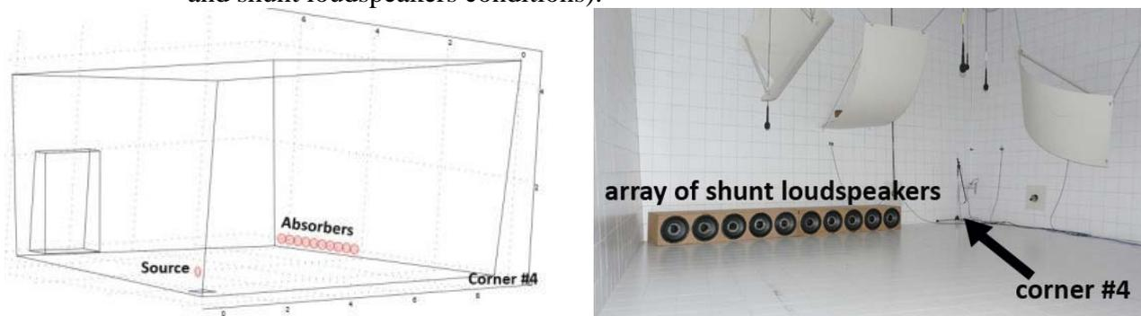
**Figure 4 : the reverberant chamber at LEMA (left: CAD model in Comsol Multiphysics®, right: photograph taken from the entrance)**
