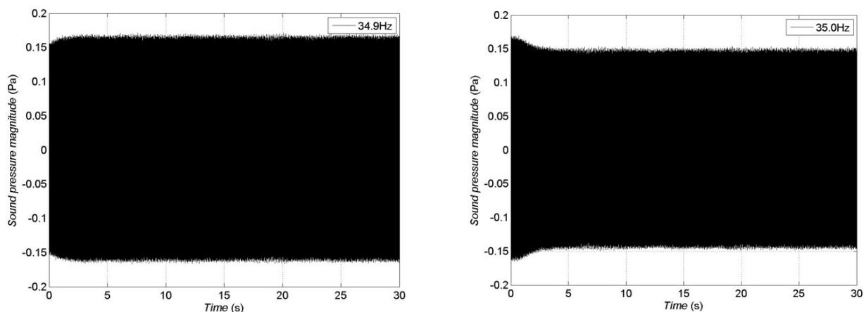
**Figure 8: temporal behaviour of the acoustic pressure in the vicinity of the mode, with 10 shunt loudspeakers (left: 34.9 Hz; right: 35.0 Hz)**
