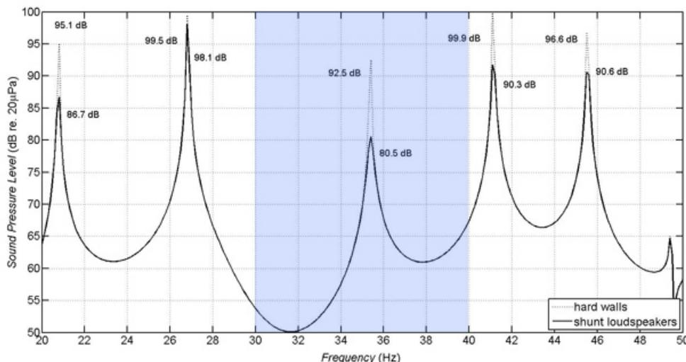
**Figure 5: Sound pressure levels computed between 20 Hz and 50 Hz, at corner 4, for different treatments (hard walls and shunt loudspeakers)**
