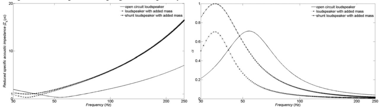
**Figure 3: computed normalized acoustic impedance  $\underline{Z}_s / \rho c$  (left) and absorption coefficient  $\alpha$  (right) of the shunt loudspeaker system**
